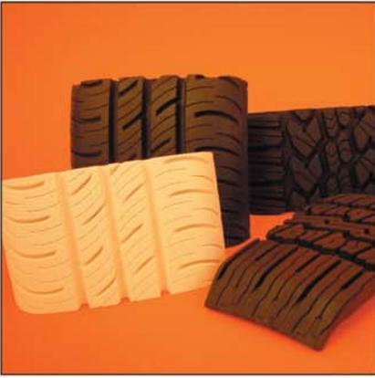
The Continental ContiProContact (left) was recently introduced in 22 sizes with advancements in wet traction and handling. The ZPrinter 310 provided the engineers with a hands-on evaluation of the tread design before investing in the expense of molds and tire building.
