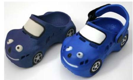
Z Corp 3D Printer prototype and final product
