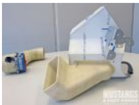
More 3D printed prototypes used for fit checks and flow testing
