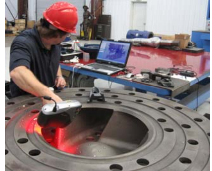
Scanning the inside of a large pump impeller with the Z Scanner 800
